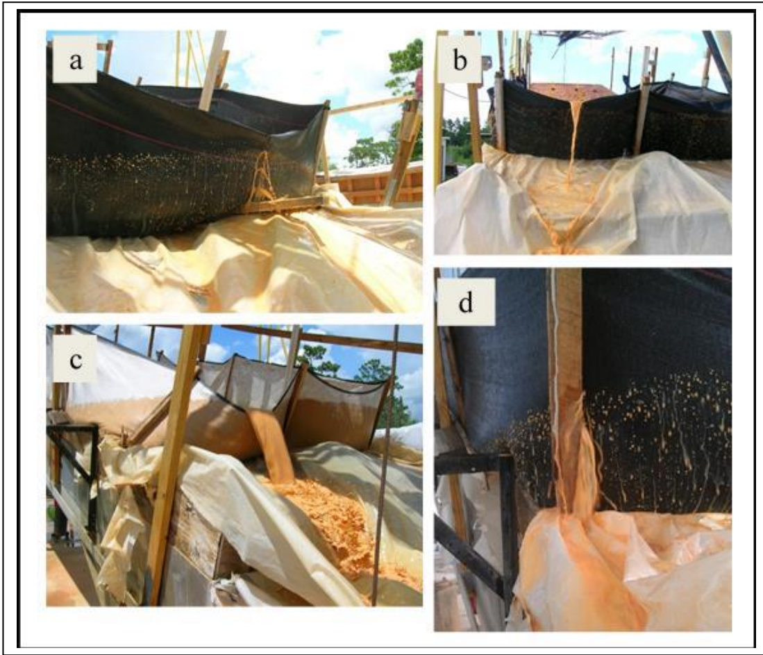
Figure 2.2-2 – Silt fence failures observed during Mr. Dubinsky’s experiments: (A) pullout of fabric from middle stake on 33% slope; (B) overtopping on 33% slope (C) corner stake failure on 33% slope; and (D) corner stake tear on 25% slope.
